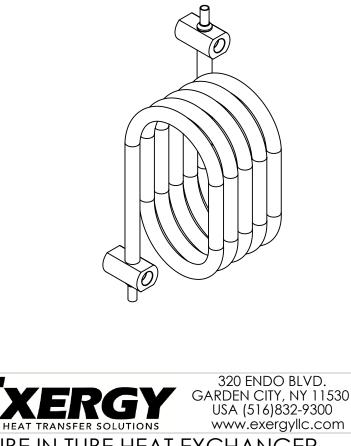
TUBE IN TUBE HEAT EXCHANGER 1.25 OUTER TUBE 3/4 TUBE STUBS MODEL NO. AS-01194 -# DATE 5/26/2023 SCALE 1:6 SHEET 1 OF 1
